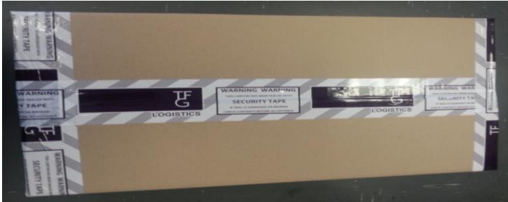
Fig 7.1: Carton to be sealed in H-Pattern on both top and bottom sides
