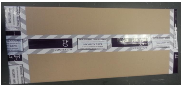
Fig 4.1: Carton to be sealed in H-Pattern on both top and bottom sides
